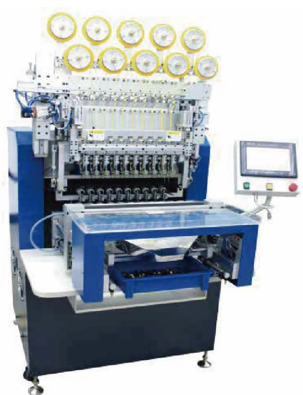
ERRS3710BD全自动绕线包胶机图 带拉包滚轮 ERRS3710BD Automatic Winding Machine with Vertical Tapping
