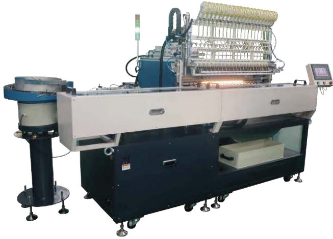
EZRS4620BAS 自动上料绕线包胶机图 EZRS4620BAS Automatic Winding Machine with Automatic Bobbin Loading and Tapping
