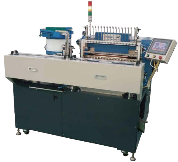
EZRS3316S 自动上料绕线机图 EZRS3316S Automatic Winding Machine with Automatic Bobbin Loading
